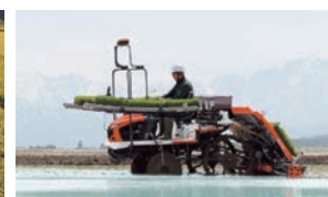
KSAS-compatible rice transplanter with an electric fertilizer volume control unit
