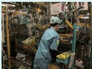
Components are provided from in front and tools are all within 40 cm of the worker, enabling them to get on with their work close at hand without twisting to look or walking around.
