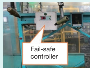
Fail-safe equipment prevents workers from forgetting to tighten bolts or applying insufficient torque. If a worker does forget, the equipment does not let them proceed to the next task.
