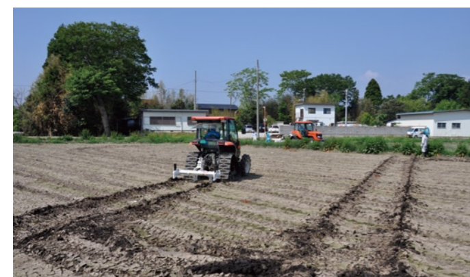
After trenching channels with a subsoiler to enhance the water's natural penetration, various types of machinery were used for different demonstration methods.
