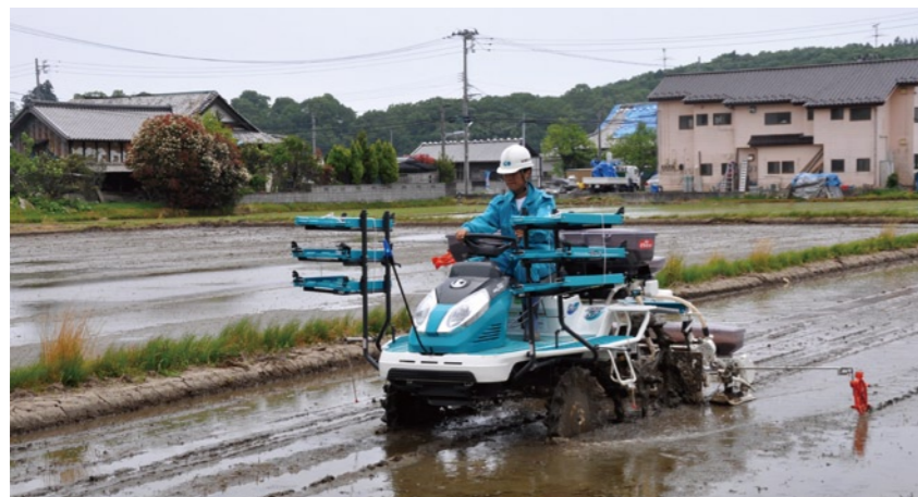
Machinery directly sows iron-coated seeds.
