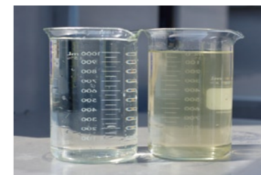
Water purified by FILCERA (left). The water can be further purified to drinking quality if the system is enhanced.
